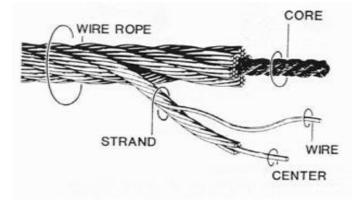
Figure 1 :Wire, Wire Rope, Strand
